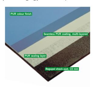
This highly resilient system is fast and responsive, designed particularly for athletic activities indoors. Its PU wear layer is 2 mm thicker than the standard version of Regugym and the base mat is 10 mm thick. Regugym SR is effectively used for multi-use facilities, field houses and indoor athletic facilities. This surface is extremely hard wearing and spike resistant.
