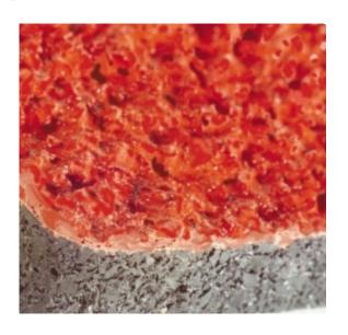
Regupol PDW is the ideal sports surface for indoor athletic facilities. Its finely granulated surface texture guarantees stability under foot. Regupol PDW consists of a prefabricated Regupol base mat fully bonded to an engineered subbase, on top of which a structural spray coating is applied in two layers. The structural spray coating is a water based polyurethane dispersion. The spray application and the components used guarantee an easy and smooth procedure.
